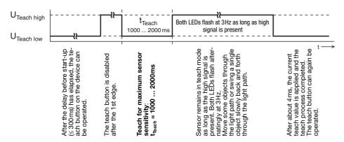
In the event of a teach error (e.g. no teach object or a teach object which is too small or too transparent is moved through the light path), the two LEDs flash at the same rate. Check the system, repeat the teach process, if necessary use a larger or less transparent teach object.
